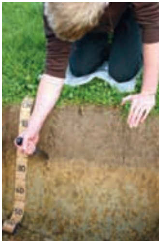
PLATE 8 Using a knife to determine the presence or absence of a hardpan
