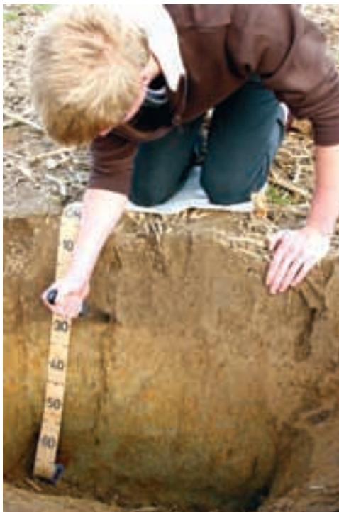
PLATE 9 Using a knife to determine the presence or absence of a hardpan
