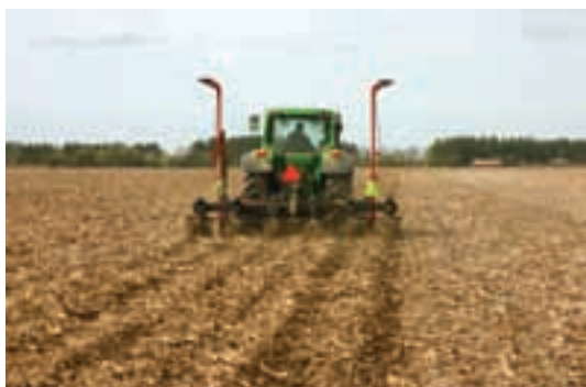
PLATE 33 Strip-tillage planting of an annual crop protected by good residue cover
