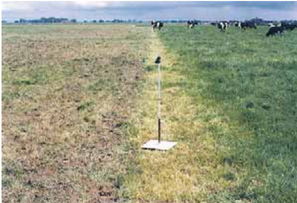
Assessing dry matter production and pasture growth rates with a rising plate meter.
