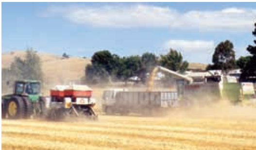
PLATE 16 Harvesting an annual grain crop followed immediately by no-till seeding the next crop into stubble [BAKER NO-TILLAGE LTD]
